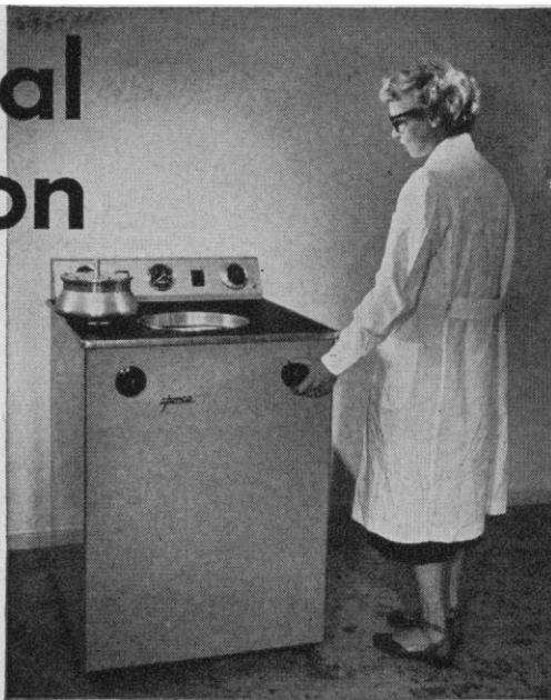
**FULLY-AUTOMATIC** features make the Spinco Model L Preparative Ultracentrifuge operationally self-supervising. Simple speed- and time-controls are preset by operator and electronic unit brings rotor to speed, times run, and decelerates with smoothly operating automatic brake.
