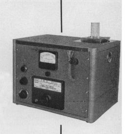
Na and K analyses in a few minutes and accurate to within 1 or 2 percent, are standard procedure with the new improved Perkin-Elmer Model 52-C Flame Photometer. Not an attachment, but a separate, *complete* installation, the Perkin-Elmer Flame Photometer operates by means of either direct intensity or internal standard methods. Analyses are readily made on blood, food, water, or any substance placed in solution. Operation is simple and dependable, results are reproducible.
