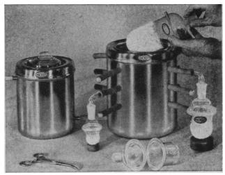
The apparatus is fitted with 12 take-off taps capable of removing a minimum of 100 ml of water.
