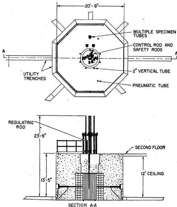
FIG. 1. General installation layout.
