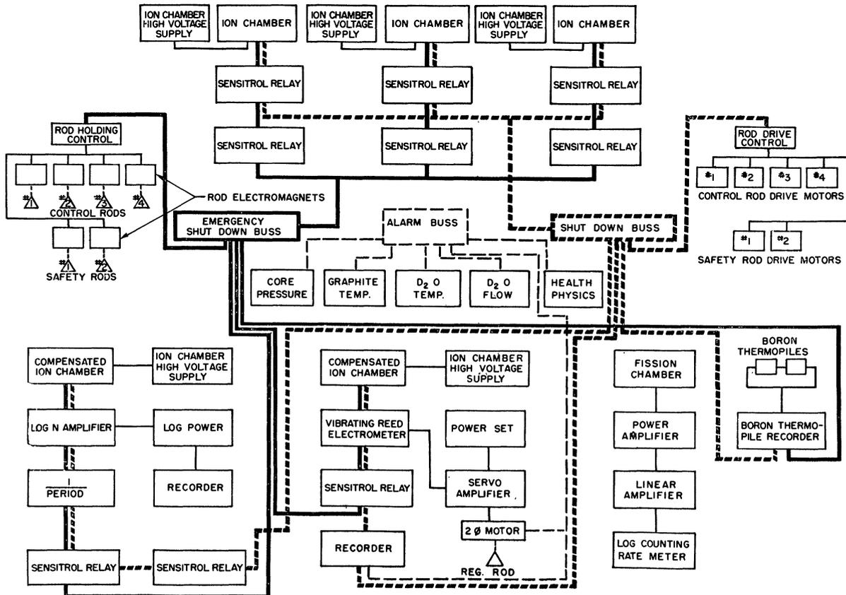
Fig. 6. Control circuit block diagram.
