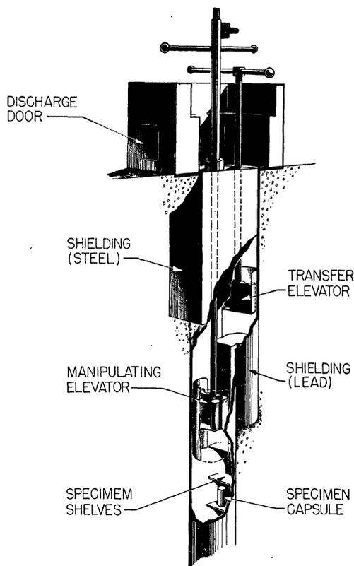
Fig. 5. Multiple specimen hole details.
