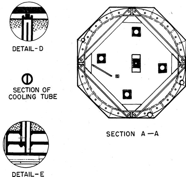
FIG. 3. Core tank details.
