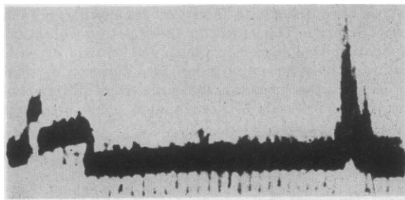
FIG. 1. Typical A-plan record of backscatter from regions to west of Sterling. Range to scattering region is shown for the instant of photographing. Transmitted pulse occurs at jog in broken rectangle at left; received echo is at right about 15 milliseconds later as shown by abscissas scale graduated in half-millisecond markers. Height of echo gives relative amplitude.
