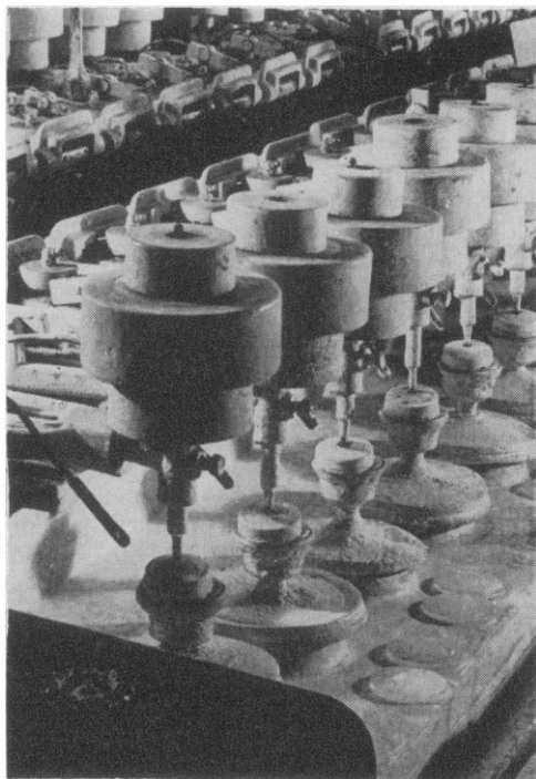
FIG. 3. Before reaching the finished state, a lens must undergo many hours of grinding and polishing.
