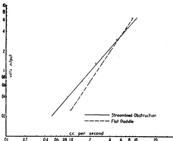
FIG. 3. Calibration curves for two flowmeters employing the 5734 tube with flat and streamlined obstructions.
