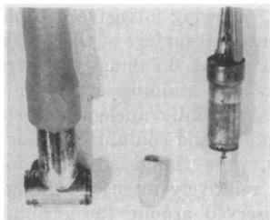
FIG. 2. A flowmeter employing the RCA 5734 tube. On the right the tube with a streamlined obstruction, in the center a flat paddle, and on the left an assembled flowmeter in stainless steel T-cannula. Diameter of the tube at its widest point is 0.375 in.
