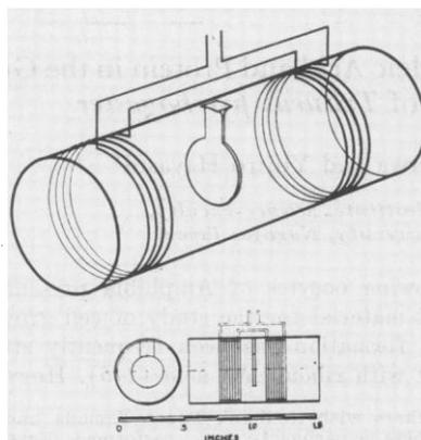
FIG. 4. Schematic diagram of a flowmeter in which a moving ferromagnetic obstruction alters the inductance of windings around a tube.
