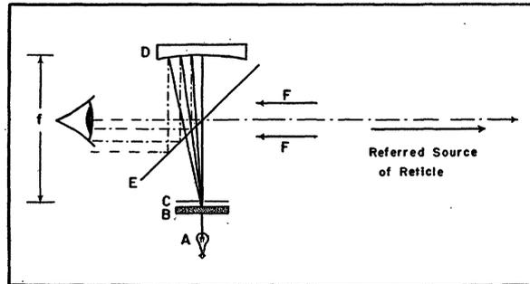
FIG. 1. Schematic diagram of a reflex sight.
