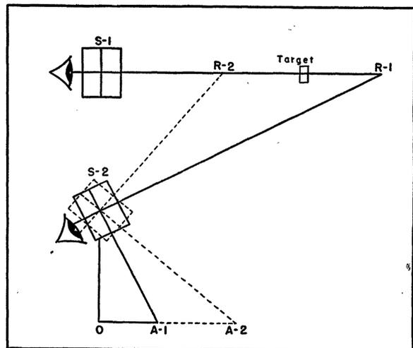
FIG. 2. Schematic diagram of a stereoptometer.
