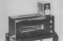
An important, new scientifically designed apparatus that determines PROTHROMBIN TIME accurately and simply. It is a completely integrated unit that eliminates variables in temperature and results. The apparatus is thermostatically controlled at 37°-38°C. and includes an electronically operated stop watch actuated by a foot switch.
