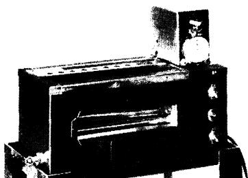
An important, new scientifically designed apparatus that determines PROTHROMBIN TIME accurately and simply. It is a completely integrated unit that eliminates variables in temperature and results. The apparatus is thermostatically controlled at 37°-38°C. and includes an electronically operated stop watch actuated by a foot switch.
