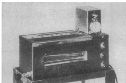
An important, new scientifically designed apparatus that determines PROTHROMBIN TIME accurately and simply. It is a completely integrated unit that eliminates variables in temperature and results. The apparatus is thermostatically controlled at 37°-38°C. and includes an electronically operated stop watch actuated by a foot switch.
