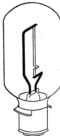
FIG. 1. General Electric ribbon filament lamp.
