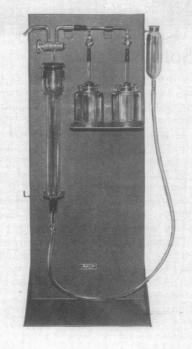
A modified Haldane gas analysis apparatus used to demonstrate the technique of gas analysis in student teaching.
