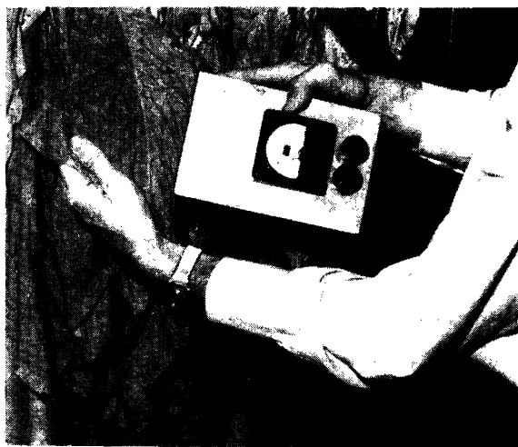
FIG. 2. Measuring reflectance of tobacco in the curing barn with the Yellowmeter.
