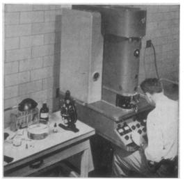
**ELECTRON MICROSCOPE**, capable of magnifying 100,000 times, is typical of the equipment available.
