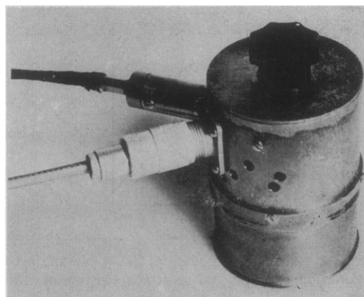
FIG. 5. The two-dimensional echoscope as used in the experiments. The flexible mechanical and electrical connections can be seen.
