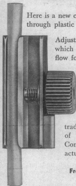
Adjusts by smooth-acting ratchet which permits minute changes of flow for infusions etc., with ready return to a former rate. One "click" equals .00078" movement of the pressure plate.
