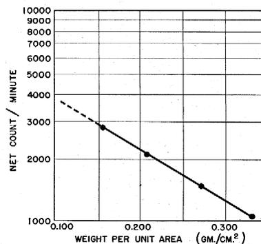
FIG. 2. Calibration curve of aluminum strips.
