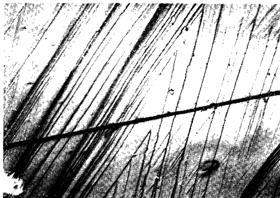
FIG. 1. Fractograph of octahedral cleavage in fluorite, revealing crystallographic features and suggesting a lamellated structure of the crystal. ( \times 175 .)
