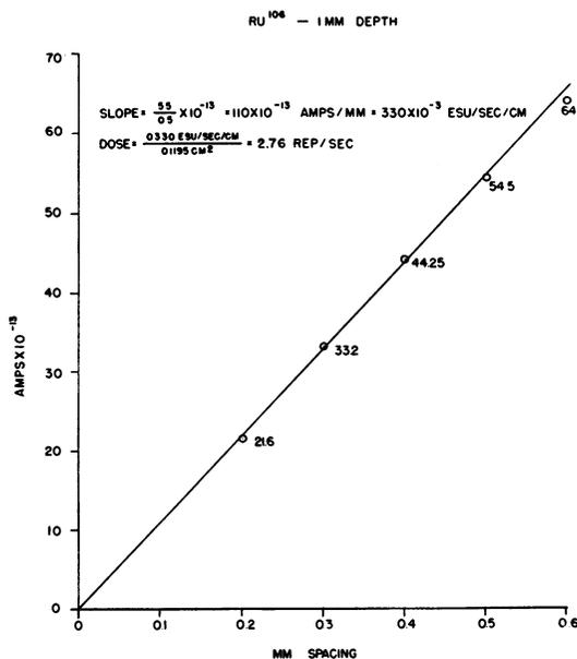
FIG. 2. Sample ionization current vs. plate spacing curve obtained using a Ru<sup>106</sup> source at 1-mm depth in a lucite phantom. Calculation of radiation dose in rep/sec for this curve is shown.
