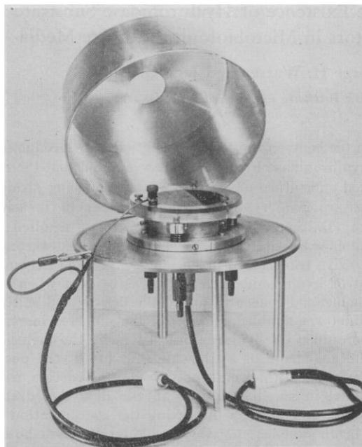
FIG. 1. Extrapolation ionization chamber.
