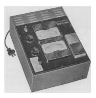
A self-contained densitometer for the accurate measurement of density of dental-size X-ray films as employed in film badge systems for personnel monitoring in radio-activity laboratories and X-ray installations
