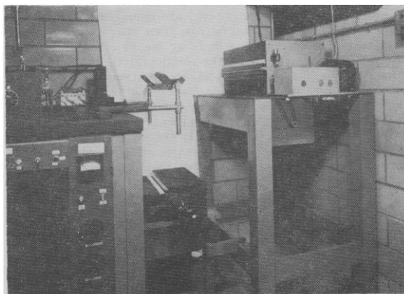
FIG. 4. Photokymographic cameras used for simultaneous recording of multiple physiologic variables concerned with the heart and circulation. Camera on the right (for 18-in. width photographic paper) is run continuously at a slow chart speed (1.25 or 5 mm/sec) throughout the procedure. The camera, mounted face up directly below the front-surfaced mirror, is set for a chart speed of 29 mm/sec and adjusted in relation to the mirror so as to photograph the lower portion of the same galvanometer beams focused on the upright camera. This fast camera is run only occasionally during the procedure, at points at which study of the contours of the recorded variations might prove of value.
