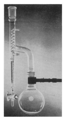
type. The reservoir, which is made from a graduated centrifuge tube, has a stopcock that permits the use of the apparatus for automatic separation of large quantities of water when a large-scale condensation is done, since an inverted  $\perp$  of rubber or glass tubing attached at the stopcock can be arranged as an automatic water takeoff. A ground joint above the spiral gives a place for an additional condenser if a very rapid reflux is needed.
