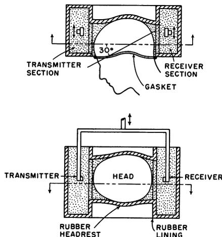
FIG. 4. Schematic diagram of tank for scanning brain of live subjects.
