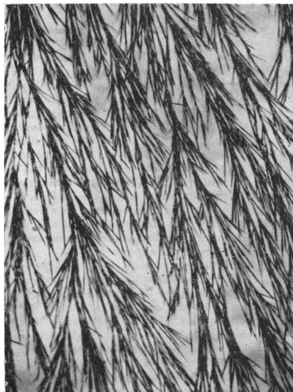
FIG. 2. Detail of structure of crystals deposited from an alcohol-ether-celloidin solution containing 1% DDT ( \times 120 ).
