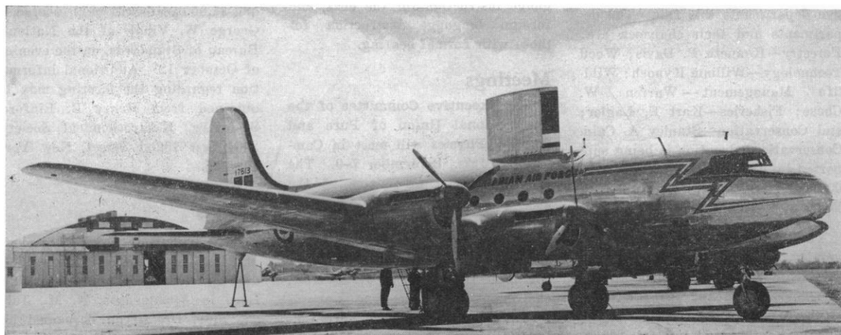
"The Rockliffe Ice Wagon," North Star plane converted by the National Research Council of Canada into a flying laboratory designed for general research on cloud physics. Flight tests will also determine the performance of experimental anti- and de-icing equipment. Most striking feature is the large "shark's fin" on top of the fuselage for use in testing the electrothermal method of wing de-icing. On either side of it are blister-type observation domes, and the propellers are fitted with blade-heater elements. J. L. Orr, head of the NRC Low Temperature Laboratory, is a member of the team of scientists that flew with the Ice Wagon to England for demonstration purposes.
