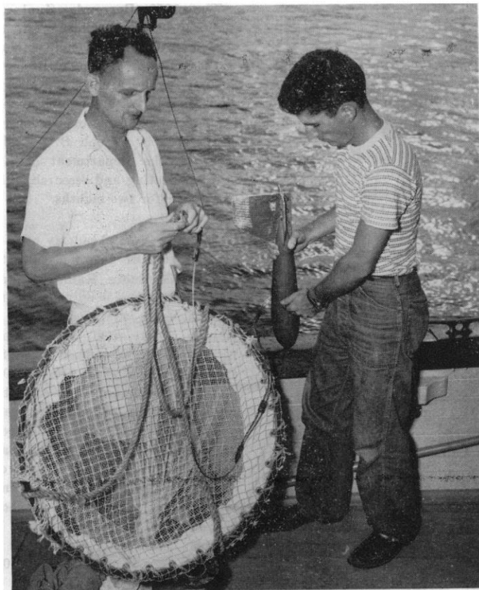
Aboard the laboratory ship Megalopa , Dr. Hilary B. Moore, associate director of the National Geographic–University of Miami plankton research expedition, helps an assistant attach a bathythermograph to the seining equipment. In addition to exploration of the ocean depths for the microscopic plankton, new information will be sought on the behavior of the Gulf Stream. Dr. F. G. Walton Smith, head of the Marine Laboratory, University of Miami, is director of the expedition, which left Miami July 25.
