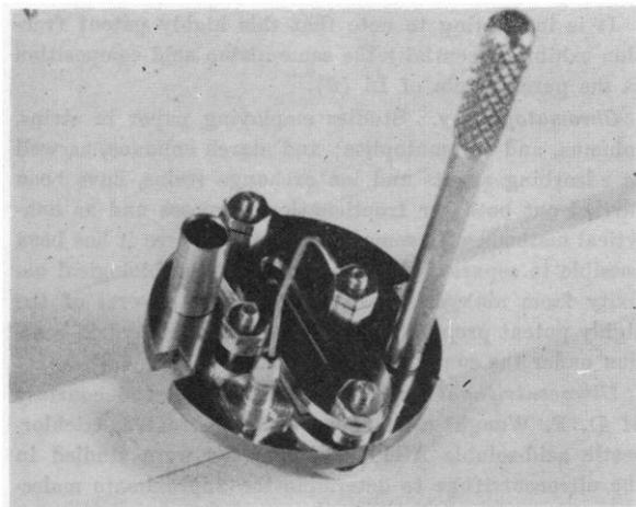
FIG. 2. Assembled absorption cell. Cell body dimensions: thickness 3.00 mm; diam 32.25 mm; front aperture 1.00 mm wide by 12.0 mm long; rear aperture 0.50 mm wide by 12.0 mm long. Window dimensions: 10 mm by 20 mm by 1 mm thick. Sample volume 25 mm<sup>3</sup>.
