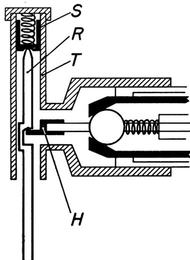
FIG. 2. T-shaped attachment to change the horizontal type micromanipulator shown in Fig. 1 to a vertical type for operations in deep holes.
