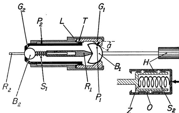
FIG. 1. A schematic cross section of the pencil-type micromanipulator. The tip, on the left, can be moved in three dimensions by moving the handle, on the right. The ratio between the magnitudes of the movements at the handle and at the tip can be set arbitrarily. Insert: Longitudinal shock absorber in the handle of the micromanipulator.
