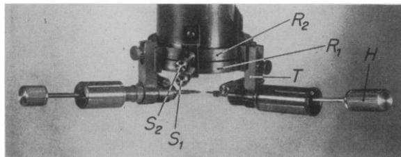
FIG. 3. Mounting for the manipulator on the objective tube of the microscope, eliminating the need for independent coarse adjustments of the manipulator.
