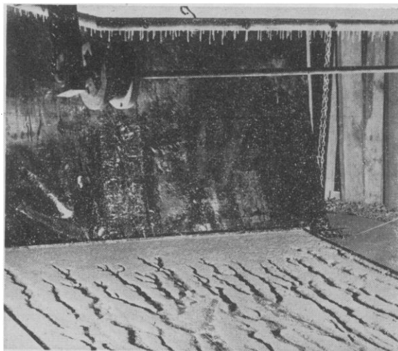
FIG. 6. Gully erosion is a product of the scour process. On this small plot the rainmaker was lowered to the surface and drops were released without impact. The soil was only about one inch deep, so that some of the washes spread in width more than they would have in deeper soil. If the raindrops had been applied with impact they would have served as a feeder agent and all of the soil would have been washed away. Soil Conservation Service photo.
