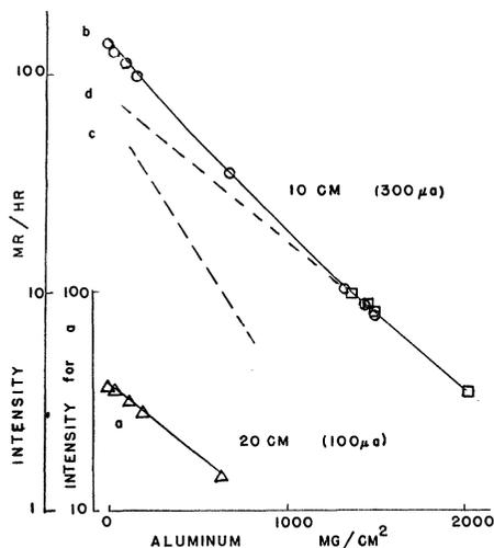
FIG. 3. Attenuation of X-rays from electron microscope.
