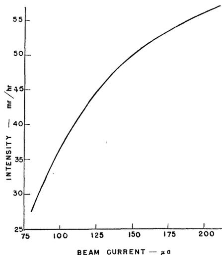
FIG. 2. Dosage vs. beam current at 20 cm.
