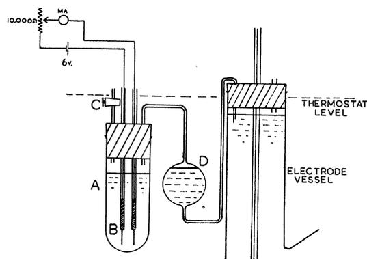
FIG. 1. Diagrammatic form of the electrolytic compensator.
