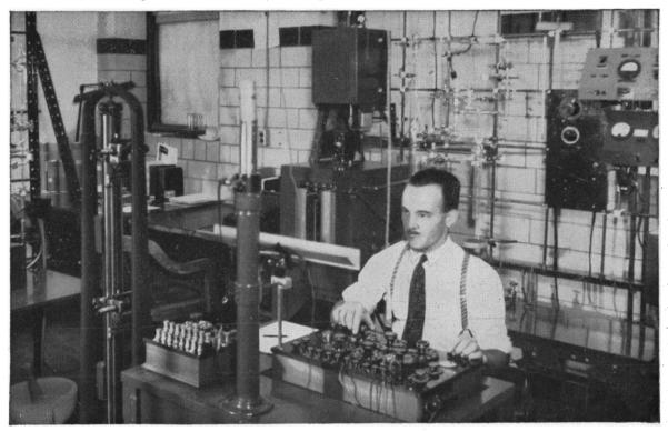
Apparatus for precise measurement of vapor pressures, photographed above and diagrammed at right, shows use of manometer, cathetometer, and G-2 Mueller Bridge at Bureau of Mines, Bartlesville, Okla. Manometer and sample container are immersed in the constant temperature bath. Before the compound to be studied is introduced into the container, the system is evacuated, using the Pirani gage to indicate pres-sure down to one micron and the ionization gage for lower pressures.
