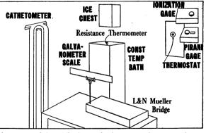
sistance of its 25-ohm platinum resistance thermometer, within a limit of error of a few tenthousandths of an ohm, or a few parts per hundred-thousand, whichever is greater.
