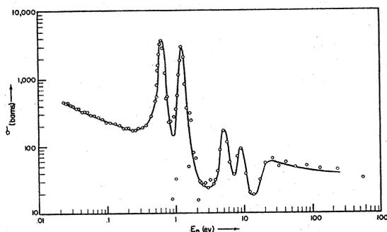
FIG. 2. The slow neutron absorption spectrum of Iridium as measured by the Columbia University neutron spectrometer group (from H. H. Goldsmith, *et al. Rev. mod. Phys.*, 1947, 19, 291). The rise to the left is typical of the  $1/v$  part of the spectrum, and the peaks are neutron capture resonances.
