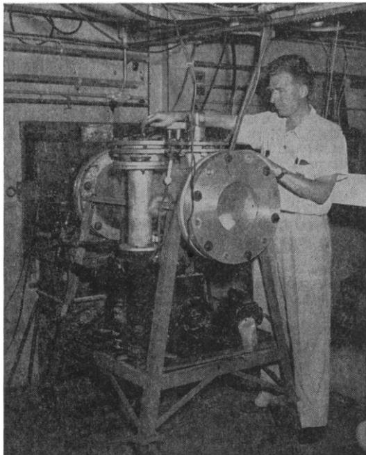
FIG. 3. Apparatus used for studying the radioactivity of the neutron. A beam of neutrons is taken from a hole in the concrete shield of the Oak Ridge reactor (background) and passes through the horizontal evacuated tank. Apparatus for counting the decay protons is inside the tank. The "bull's-eye" on the end of the tank is the thin aluminum window through which the beam emerges, to be caught finally in a heavy boron-laden, lead-shielded "beam-catcher" 10' away.
