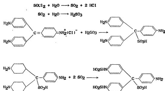
FIG. 1. Reactions which can be expected to occur when thionyl chloride is used as a source of sulfurous acid in Schiff's reagent.
