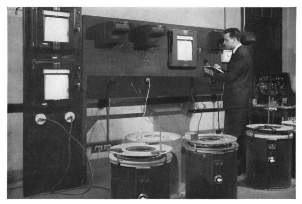
Metallurgist at University of Notre Dame transcribes temperature data from four-point Speedomax Recorder connected to furnaces in foreground. Experiment is part of
