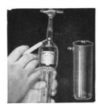
The reliable, sinking-ball valve automatically controls gas flow with a minimum of stopcock manipulation.
