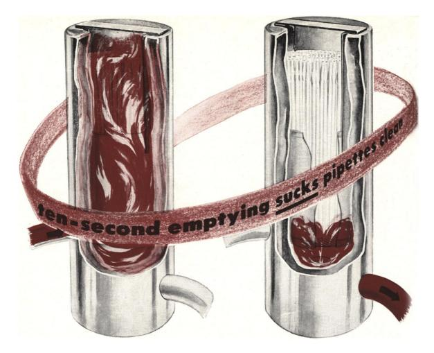
Twice every minute the TECHNICON Pipette Washer completes its syphon-cycle... seven surging gallons of water to loosen and dislodge clinging residues. Wastes are then literally swept out of the pipettes by the violent suction set up during the brisk ten-second emptying phase.
