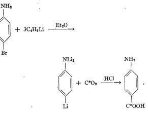
A reaction using 3 millimols of ordinary  $BaCO_3$  has resulted in a 21 per cent yield of p-aminobenzoic acid of high purity.
