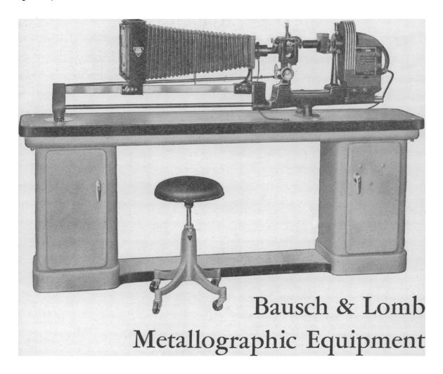
Whether it is to be used for visual observation or the photography of metal, the Bausch & Lomb ILS Metallographic Equipment provides an instrument easily adaptable to meet the major demands of metallography.
