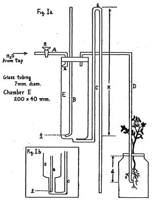
more effective gas distribution at the terminal end of the aeration tube, D. However, it has been determined that a low porosity tube introduces some difficulty. The magnitude of the frictional resistance to gas flow offered by such material results in an undesirable increase in the total pressure which must be exerted by the expanding gases in E to overcome the gross resistance in the system.
