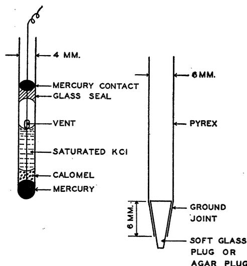
FIG. 1. Details of construction of the microcalomel electrode.
