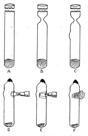
A noticeable advantage is the fact that the cotton plug is protected by the glass walls of the funnel, and only unusual handling will cause the fluid in the tube to come in contact with the cotton.
