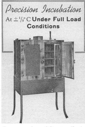
A constancy of  $\pm 1/5^{\circ}$  C. and a uniformity of  $\pm 7/8^{\circ}$  C. under full load conditions characterizes the performance of the Castle Precision Incubator No. 554. This is far in excess of the tolerance of  $\pm 1^{\circ}$  C., recommended by the American Public Health Association.
