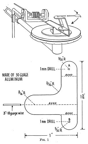
wire. The figure shows the pattern for the carrier. The metal when thus shaped is folded over one end of the 18-gauge wire and crimped so as to hold. The wire is then placed in the spindle in the same manner as the old lever wire. The old writing arm is cut to the desired length and about one-half inch bent to nearly a right angle. The short arm of this right angle is inserted in the holes A and B, as shown in
