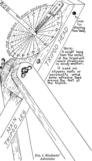
may be accurately placed by orienting it with a magnetic compass with due allowance for compass declination, and by using a plumb bob to get the right slant, as suggested in the picture for a station in the latitude of New York. The plumb bob consists of a small weight supported by a thin thread which is held in a slit on the degree mark on the declination disk corresponding to the latitude of the place.
