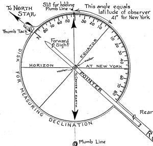
so that the long rod, or right ascension axis, can be pointed at the North Star. This is done by sighting through the eyelets on the pointer, which is first set in the position shown. The declination disk is securely fastened to a flattened side of the long rod, the lower end of which passes through the right ascension disk and rests on a hole bored in the tripod head. The small indicator close to the right ascension disk is set in a plane parallel to the declination disk.
