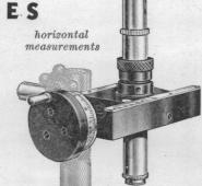
A most desirable feature of these instruments is the diversity of applications possible. In addition to the uses indicated, displacements on small objects can be measured by mounting them directly on the slide. Two slides can be mounted to form a small coordinate comparator. Etc., etc.
