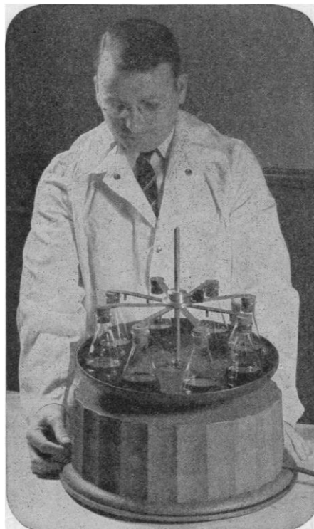
The Gyrosolver agitates as many as twelve flasks simultaneously: it holds containers up to 1,000 ml. capacity.
