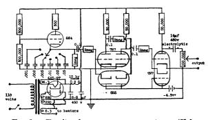
FIG. 1. Circuit of square-wave generator. (Values are not critical.) The 100,000 ohm output potentiometer should be tapered as for an audio gain control.
