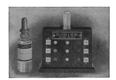
Two simple outfits for swimming pool control. Model C, for chlorine control only, contains 6 standards 0.0, 0.1, 0.2, 0.3, 0.5, 0.8 ppm. Model A, for both pH and chlorine, contains 4 chlorine standards 0.1, 0.3, 0.5, 0.8 ppm and 4 phenol red standards 6.8, 7.2, 7.6, 8.0, Sets include test cell, vial of reagent and pipette.
